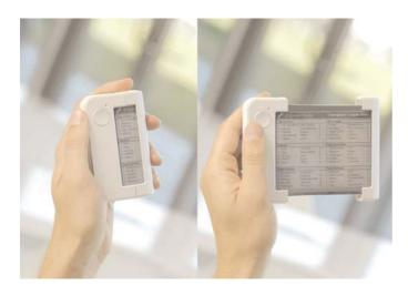
Polymer Vision's READIUS $^{TM}$  can unroll its display to a scale larger than the device itself. (Courtesy of Polymer Vision / Philips).
