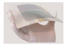
Processing of low-temperature poly-silicon (LTPS) on metal foil (courtesy of CEA-LETI)
